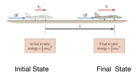
Difference in kinetic energy = Final kinetic energy - Initial kinetic energy.
