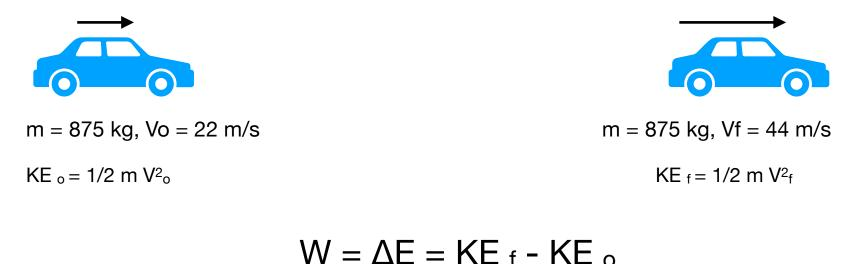
$$W = \Delta E = 1/2 \text{ m V}_{f}^2 - 1/2 \text{ m V}_{o}^2$$
