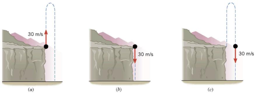
(a) From the edge of a cliff, a pellet is fired straight upward from a gun. The pellet's initial speed is 30 m/s. (b) The pellet is fired straight downward with an initial speed of 30 m/s. (c) Another representation of (a) that is based on symmetry.
