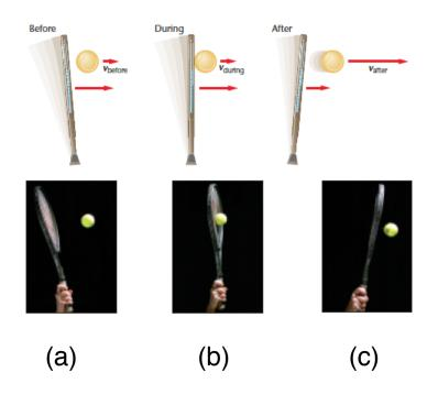
During this process, the force (F) of the racquet increases to a maximum then decreases to zero during an interval of time  $\Delta t$  as shown in the figure below:
