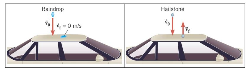
The raindrop comes to a stop (final velocity  $V_f = 0$  m/s), while the hailstone changes its velocity from  $V_o$  downward to  $V_f$  upward. Therefore, the change in momentum for the hailstone is greater. Consequently, a greater impulse acts on the hailstone. The car roof experiences a greater force. (*Action-Reaction*)
