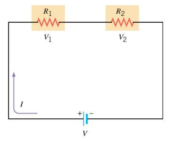
Equivalent Voltage and Resistance in Series Circuit
