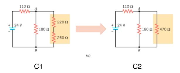
The two series resistors 220 and 250  $\Omega$  in C1 can be replaced by an equivalent resistor of 470  $\Omega$  in C2.
