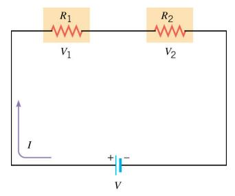
Equivalent Voltage and Resistance in Series Circuit
