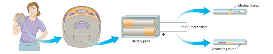
"Electron Flow" current is what constitutes an electric current in a solid conductor (such as wire). It is the flow of negatively charged electrons from the negative terminal to the positive terminal of the source of electric potential.
