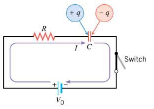
**Example 3**; Capacitor Discharging: Circuit Schematic;
