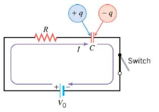
**Example 3**; Capacitor Discharging: Circuit Schematic;
