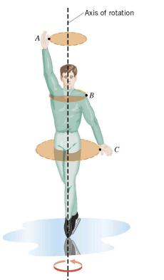
In this figure of a skater, all the points of his body such as A, B, and C circulate around the axis of rotation. He is spinning in a rotational motion.
