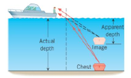
Similarly, looking directly above the object at an actual depth d, the object appears closer at an apparent depth of d'.
