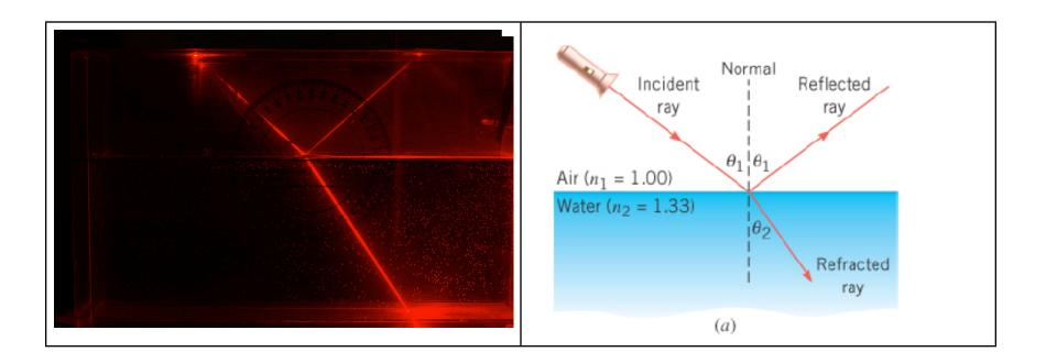
Partial Reflection: Part of the light is reflected. The angle of incidence and the angle of reflection are equal ( $\theta_1$ ).
