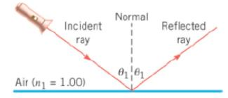
The angle of incidence is the angle between the incident ray and the normal at the point of incidence. The angle of reflection is the angle between the reflected ray and the normal.
